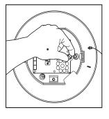
b. Turn the thumb screw and open the hinged door to the back box. Pull wiring into the back box through the conduit fitting.
